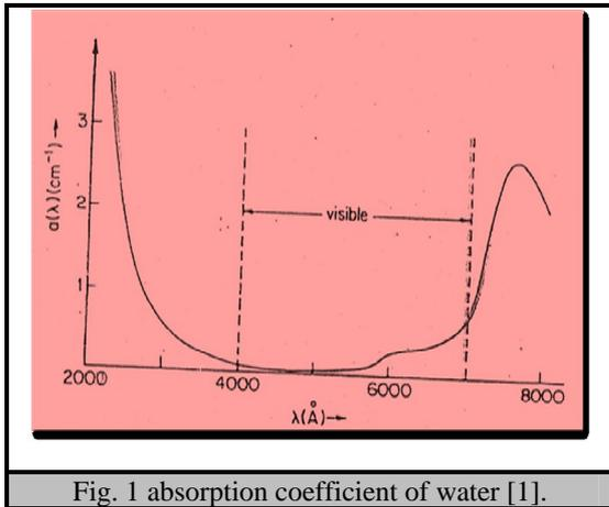
Fig. 1 absorption coefficient of water [1].
