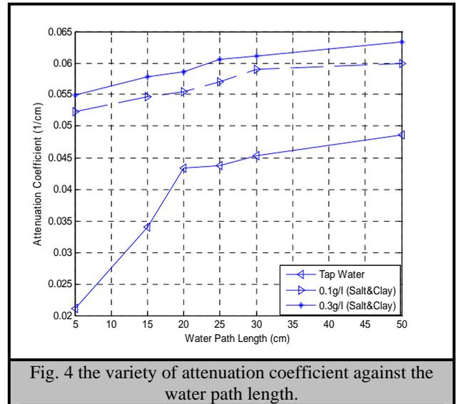
Fig. 4 the variety of attenuation coefficient against the water path length.
