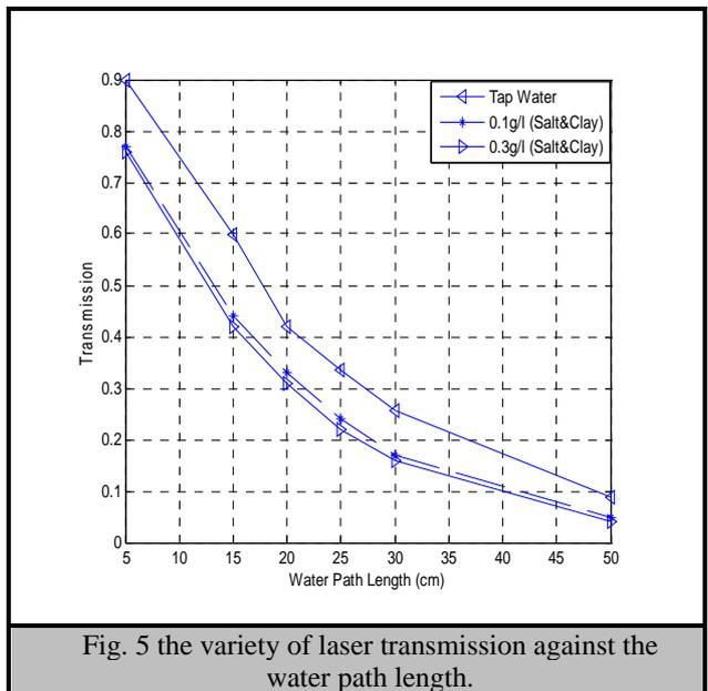
Fig. 5 the variety of laser transmission against the water path length.
