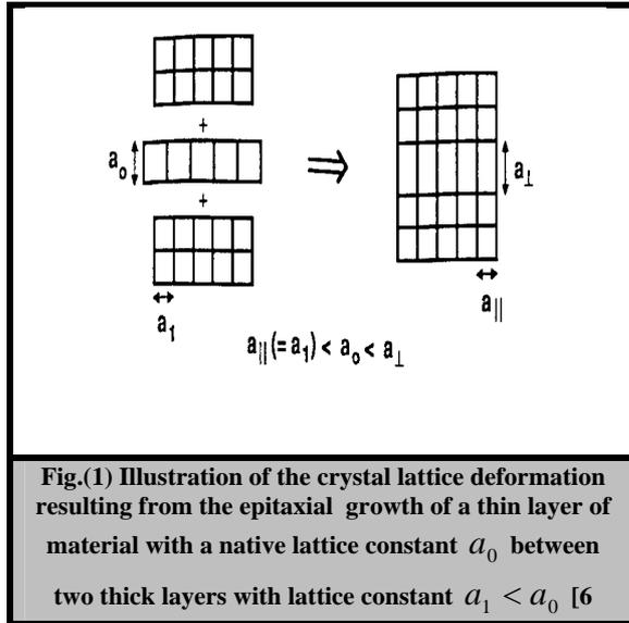
**Fig.(1) Illustration of the crystal lattice deformation resulting from the epitaxial growth of a thin layer of material with a native lattice constant  $a_0$  between two thick layers with lattice constant  $a_1 < a_0$  [6**
