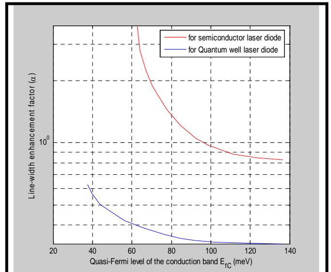
Fig. 5 Spectral line-width enhancement factor as a function of Quasi-Fermi level of conduction band
