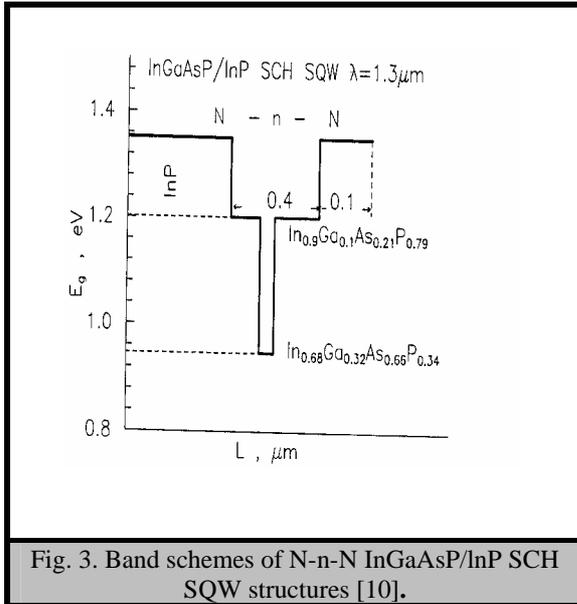
Fig. 3. Band schemes of N-n-N InGaAsP/InP SCH SQW structures [10].
