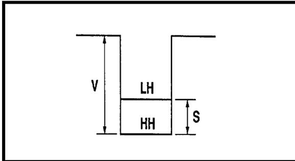
Fig.2 The modified potential barrier of a quantum well, when the well material is under compressive strain [2].
