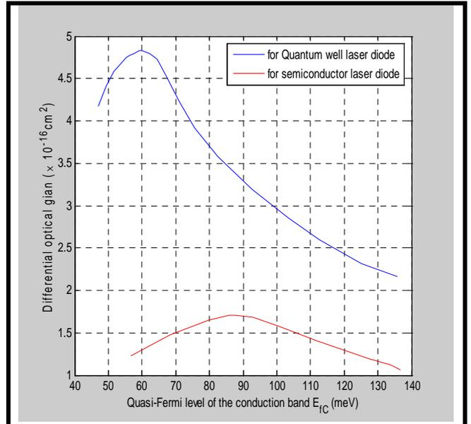
Fig. 4 Differential optical gain variation with Quasi-Fermi level of the conduction band
