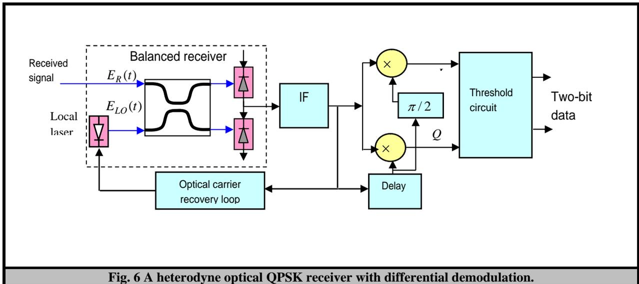
Fig. 6 A heterodyne optical QPSK receiver with differential demodulation.
