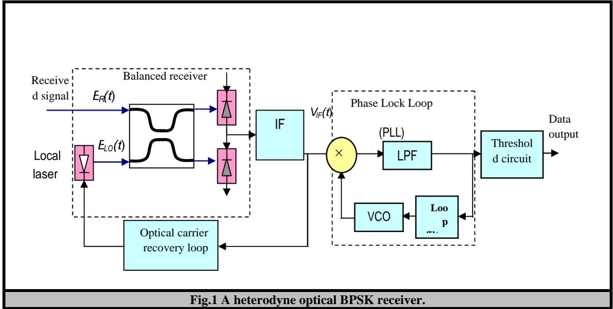
**Fig.1 A heterodyne optical BPSK receiver.**
