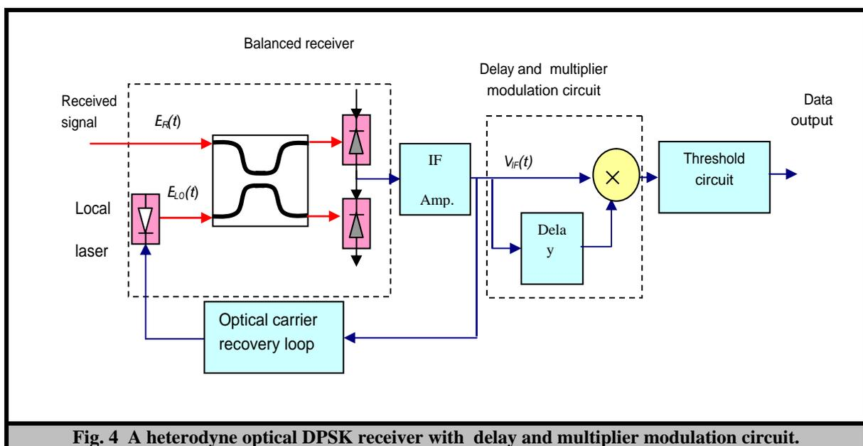
Fig. 4 A heterodyne optical DPSK receiver with delay and multiplier modulation circuit.
