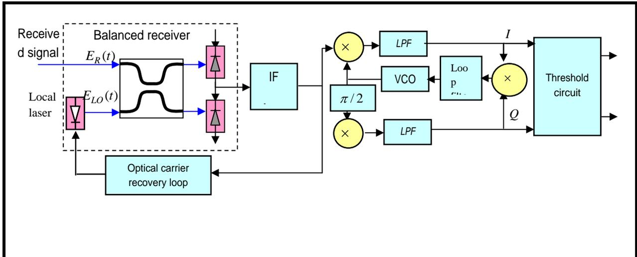
Fig. 5 A heterodyne optical QPSK receiver with coherent demodulation.
