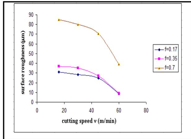
Fig. (2) - Relationship between cutting speed and Surface roughness fore cast iron
