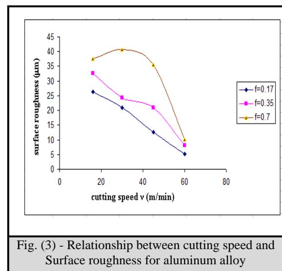
Fig. (3) - Relationship between cutting speed and Surface roughness for aluminum alloy
