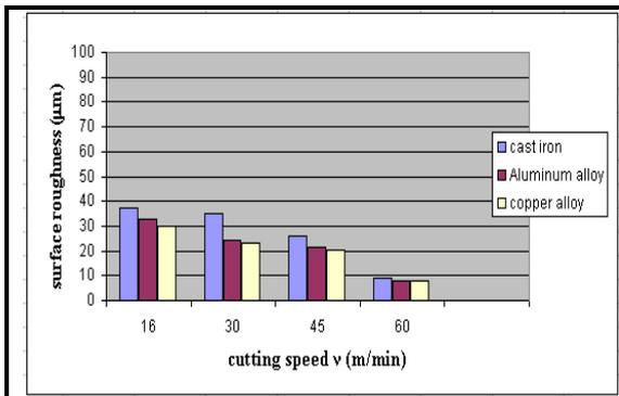
Fig. (6) - The relation between  $v$  and  $R_z$  for three materials at  $f = 0.35$  mm/rev
