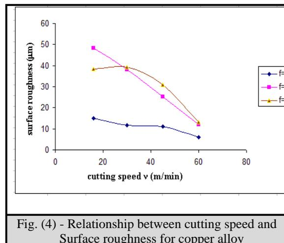
Fig. (4) - Relationship between cutting speed and Surface roughness for copper alloy
