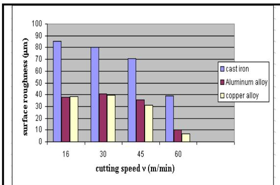
Fig. (7) - The relation between  $v$  and  $R_z$  for three materials at  $f = 0.7$  mm/rev
