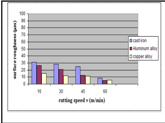
Fig. (5) - The relation between  $v$  and  $R_z$  for three materials at  $f = 0.17$  mm/rev
