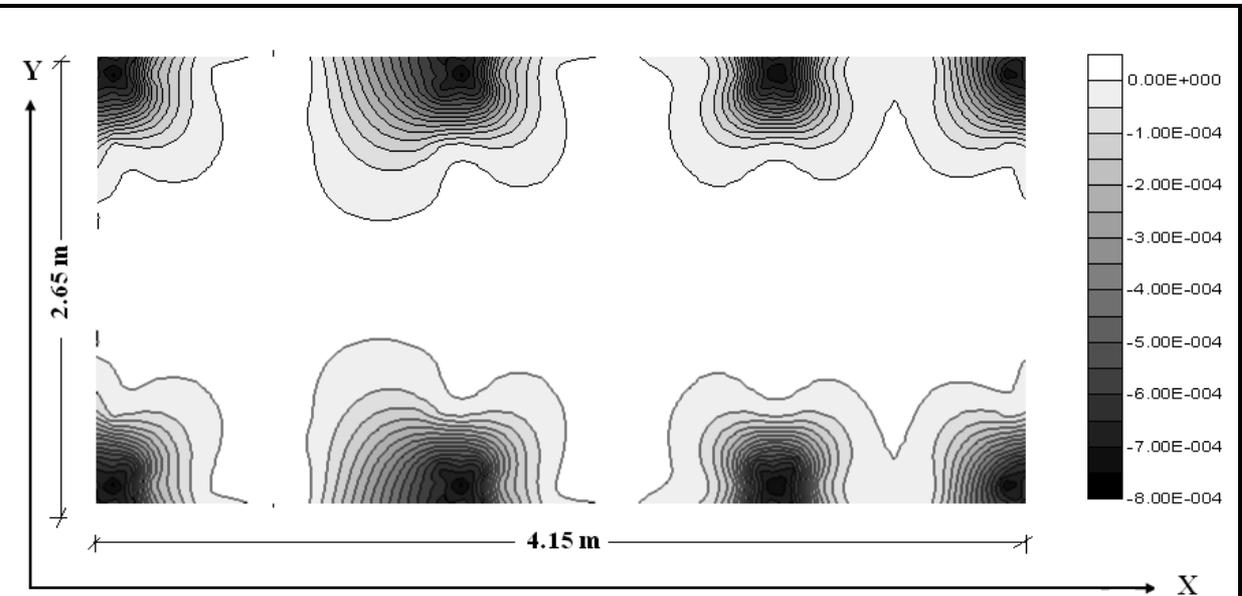
**Figure (6): Horizontal principal tensile strain at the bottom of asphalt layer ( $\epsilon_r$ ) ( $t_1=7.6$  cm and  $t_2=56.6$  cm).**
