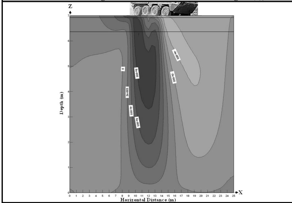
Figure (10): Vertical strain ( $\epsilon_v$ ) due to braking force combined with vehicle weight of CM32 four-axle as shown in Figure (8).
