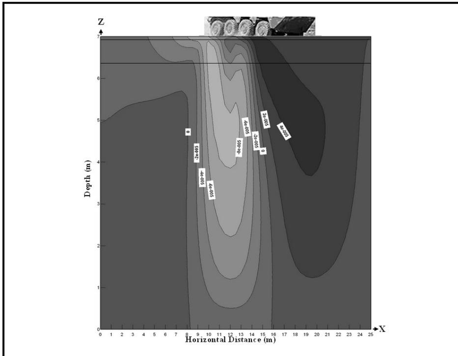
Figure (9): Horizontal principal tensile strain ( $\epsilon_r$ ) due to braking force combined with vehicle weight of CM32 four-axle as shown in Figure (8),
