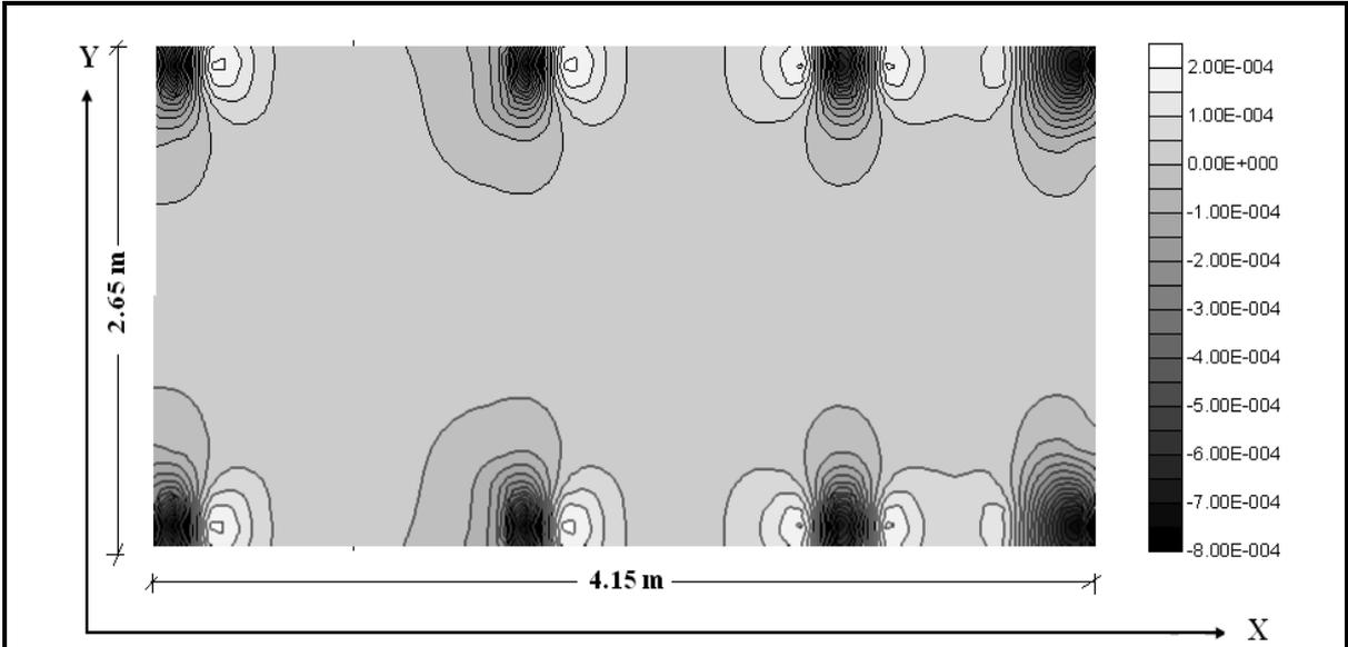
Figure (4): Tensile strain in the x direction ( $\epsilon_x$ ) at the bottom fiber of asphalt layer ( $t_1=7.6$  cm and  $t_2=56.6$  cm).
