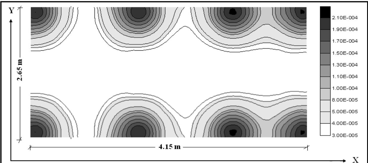
Figure (7): Vertical strain in the z direction ( $\epsilon_z$ ) on the surface of sub-grade layer ( $t_1=7.6$  cm and  $t_2=56.6$  cm).
