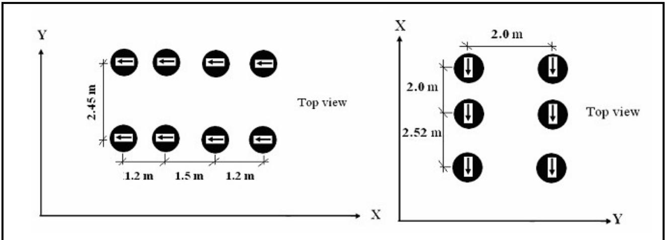
Figure (8): The layout of braking forces of four-axle and triple-axle military armored vehicles on the pavement for analysis purposes.
