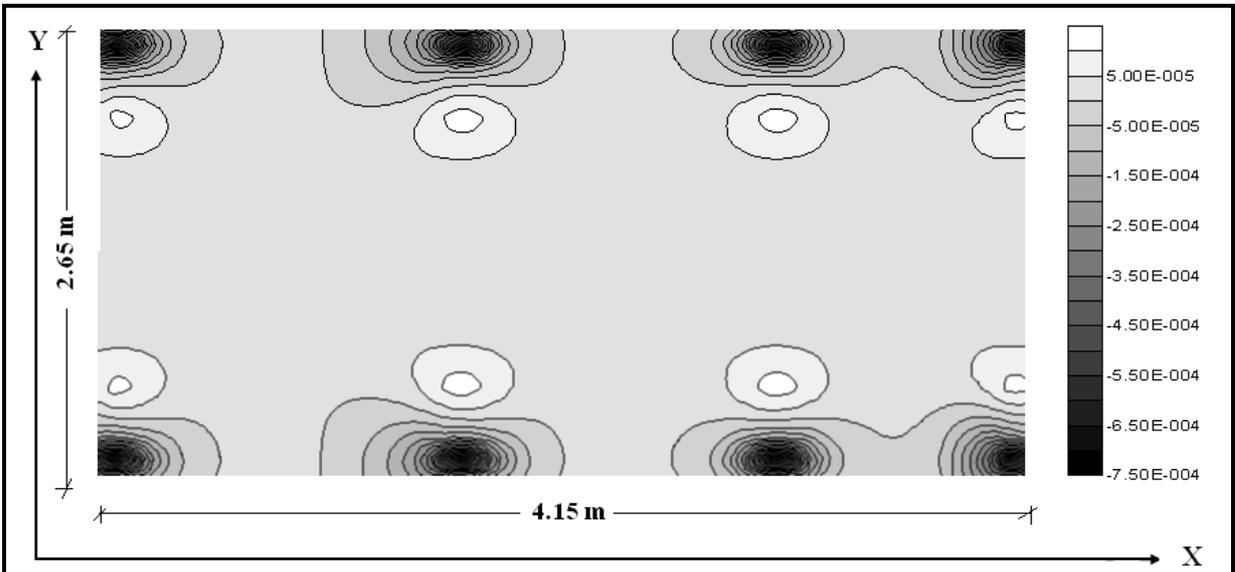
**Figure (5): Tensile strain in the y direction ( $\epsilon_y$ ) at the bottom fiber of asphalt layer ( $t_1=7.6$  cm and  $t_2=56.6$  cm).**
