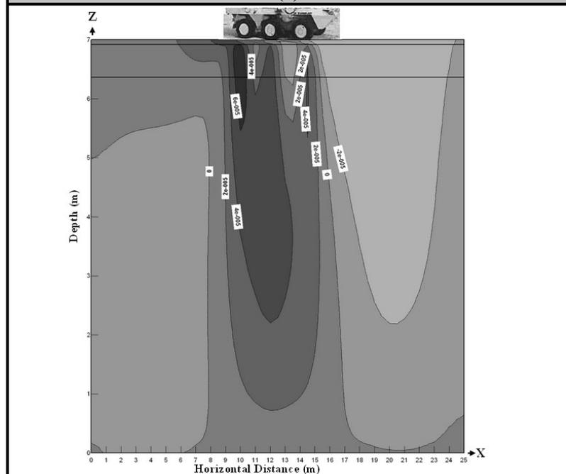
**Figure (12): Vertical strain ( $\epsilon_v$ ) due to braking force combined with vehicle weight of CM32 triple-axle as shown in Figure (8).**
