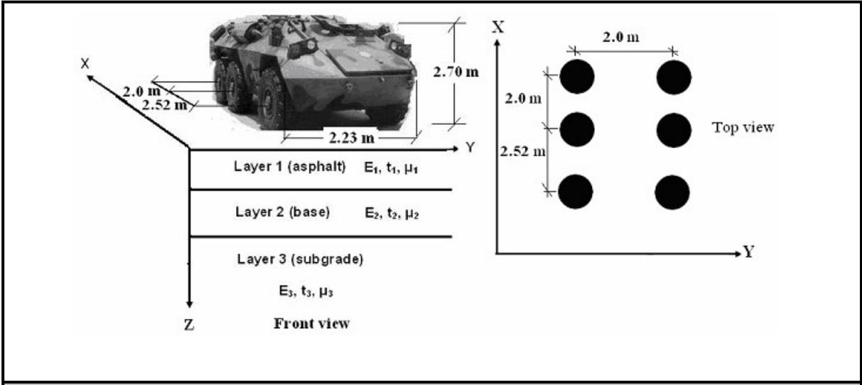
Figure (3): CM32 triple-axle armoured vehicle with rubber tiers
