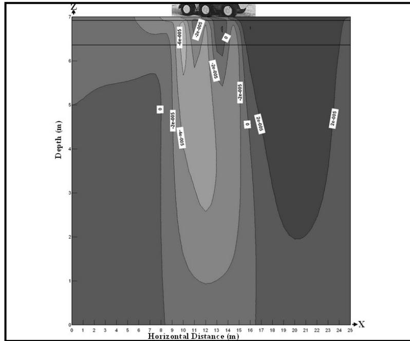
**Figure (11): Horizontal principal tensile strain ( $\epsilon_r$ ) due to braking force combined with vehicle weight of CM32 triple-axle in Figure (8).**
