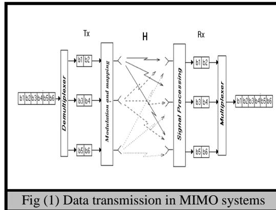
Fig (1) Data transmission in MIMO systems
