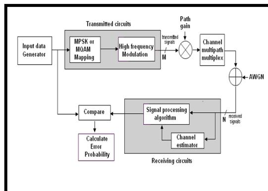
**Fig (3)** Block diagram for system Simulations
