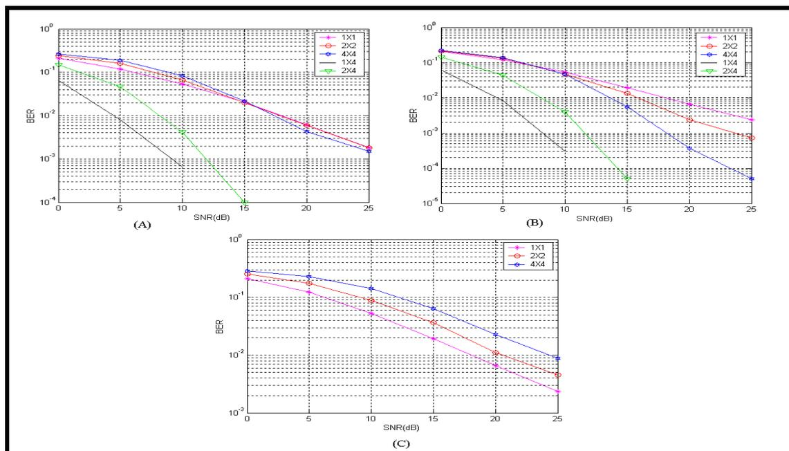
Fig.6 : BER vs. SNR, Rayleigh Fading, 4PSK modulation, with different No.of antennas.
