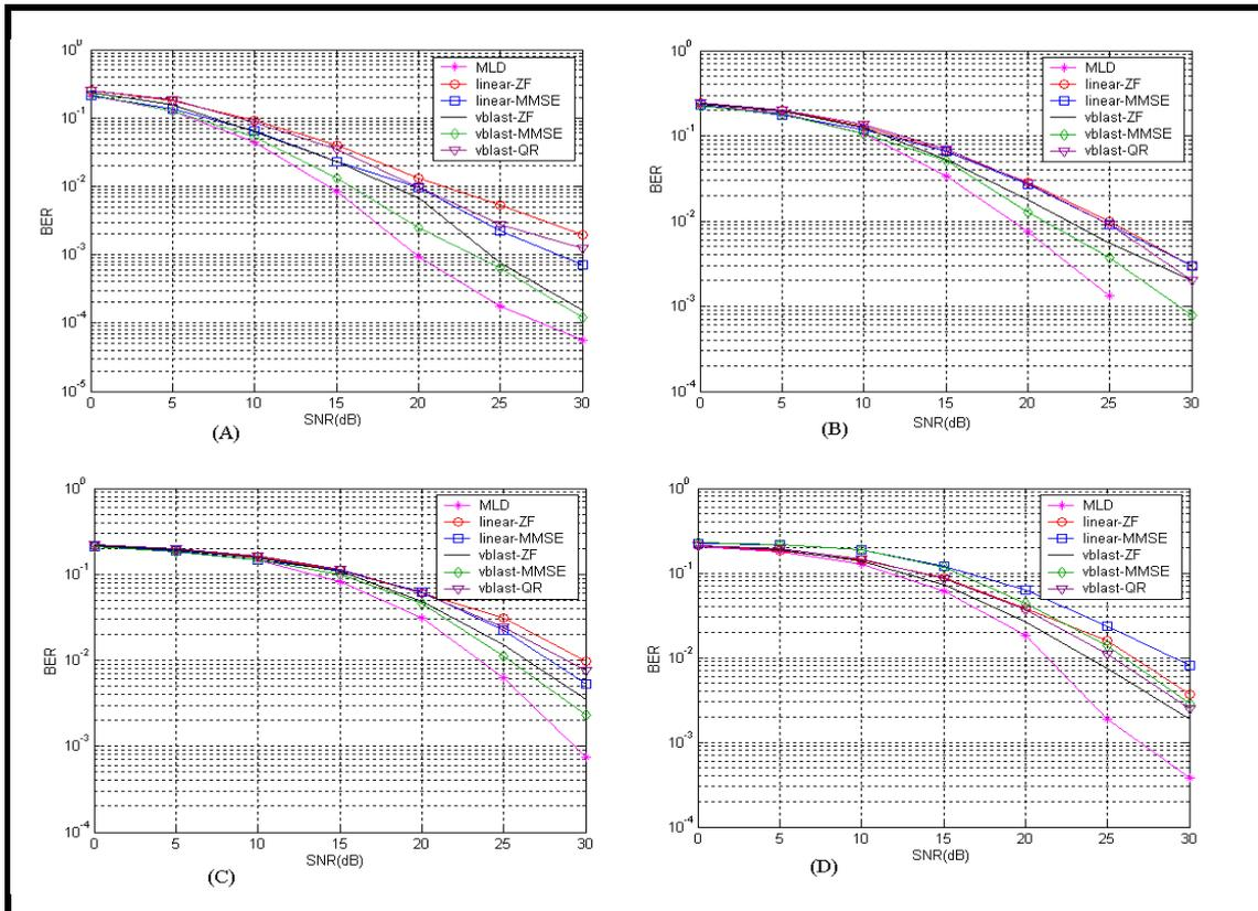
Fig. 5: BER vs. SNR, using Rayleigh fading , for all receiver types, with (2X2) antennas.
