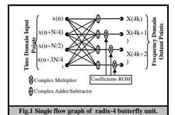
Each butterfly requires four complex adder/subtractors and three complex multipliers. The mathematical model for each radix-4 butterfly is:
