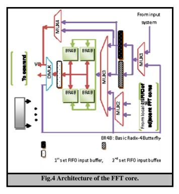
As mentioned above, the result of the BR4B is stored in local 16FIFO buffer and then sent to one of the storage sources depending on which stage is being executed as shown figure 2 and figure 4.
