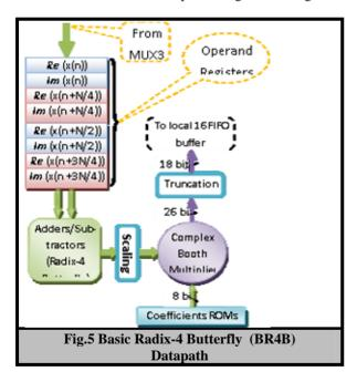
The scaling of the intermediate results in FFT computation is necessary in order to prevent overflows which can be handled in three ways[22]:
