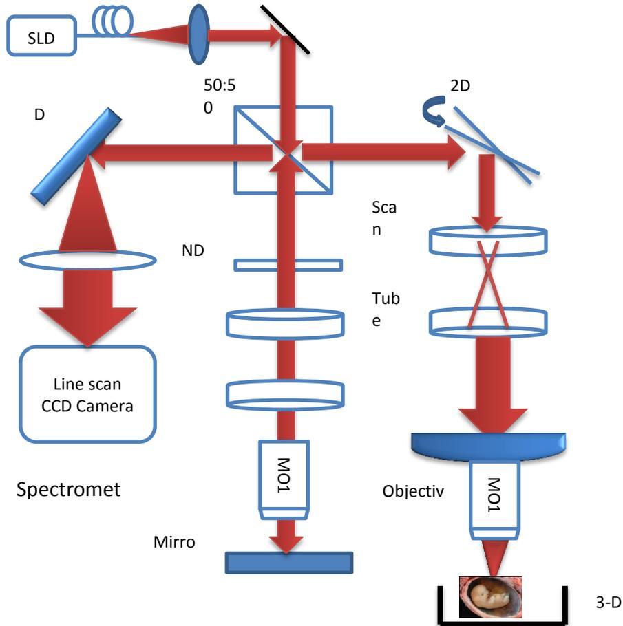
**Figure 1:** Schematic setup OCM microscope, built for *in vivo* imaging of chick and mouse embryonic heart.
