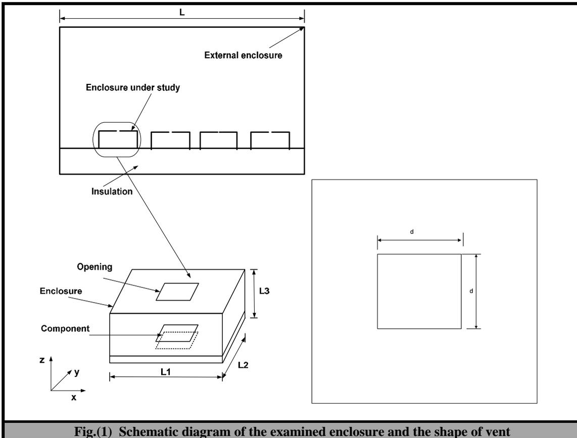
Fig.(1) Schematic diagram of the examined enclosure and the shape of vent
