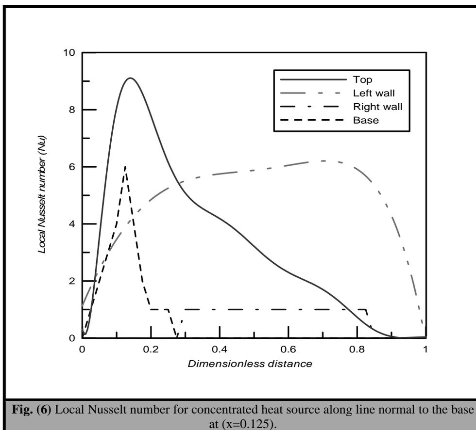
Fig. (6) Local Nusselt number for concentrated heat source along line normal to the base at ( $x=0.125$ ).
