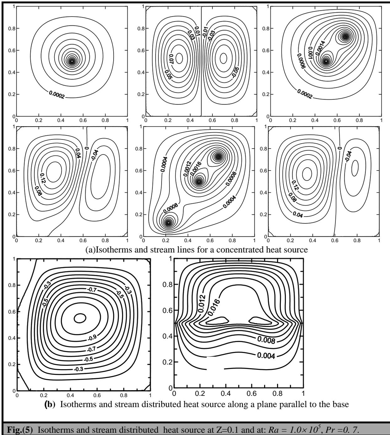
rotating-rolls. There are two high temperature regions in both left and right sides; and adjacent to the heat source position. The major of the heat is accumulated at the upper face of the heat source and decay rapidly near the walls. There is one high temperature region near the right end of the heat source. The distance between the high temperature region and the right side of the enclosure, decreases as the heat source for point or line
