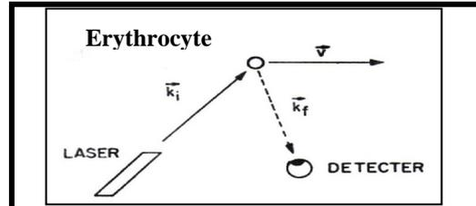
**Figure 1.** Schematic diagram of the scattering of laser light by a moving erythrocyte.
