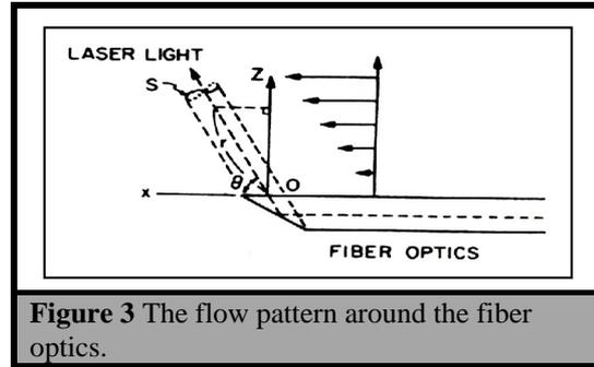
Figure 3 The flow pattern around the fiber optics.
