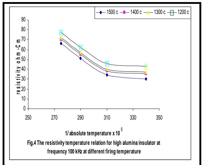
Fig.4 The resistivity temperature relation for high alumina insulator at frequency 100 kHz at different firing temperature
