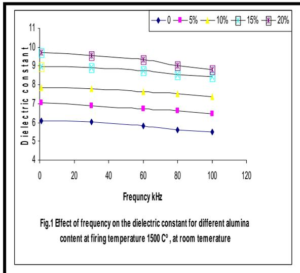
Fig.1 Effect of frequency on the dielectric constant for different alumina content at firing temperature 1500 C°, at room temperature
