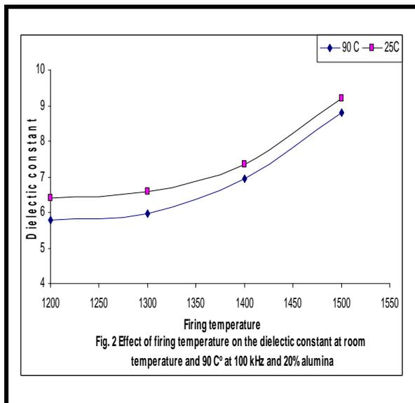
Fig.2 Effect of firing temperature on the dielectric constant at room temperature and 90 C° at 100 kHz and 20% alumina
