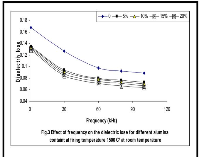
Fig.3 Effect of frequency on the dielectric loss for different alumina content at firing temperature 1500 C° at room temperature
