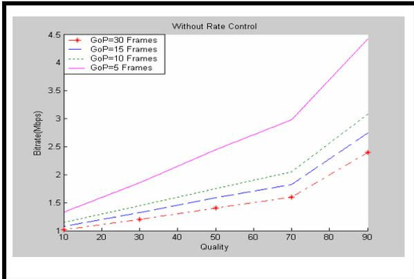
Figure (5) Bit rate versus the different quality
