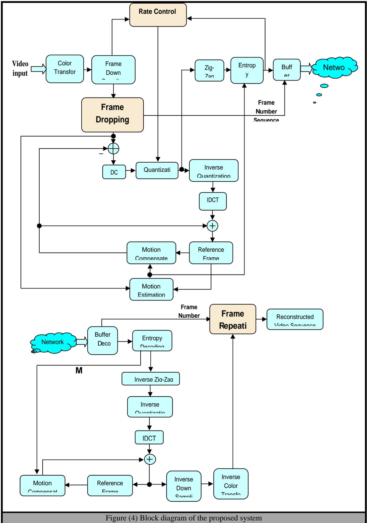
Figure (4) Block diagram of the proposed system
