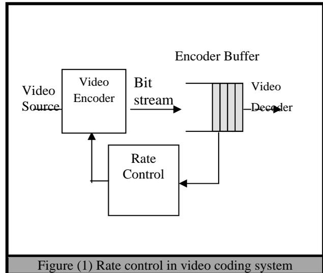
Figure (1) Rate control in video coding system
