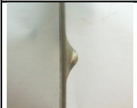
**Figure 6-3** The bulge height for biaxial compression case ( $F=0.6F_{Buckling}$ ) at  $V_i = 400$  m/s
