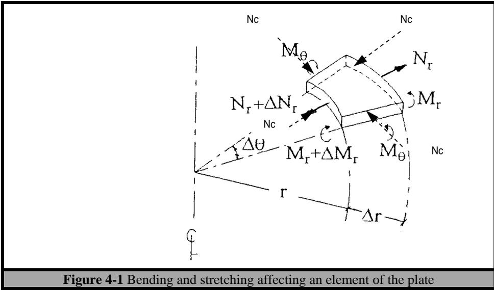
Figure 4-1 Bending and stretching affecting an element of the plate
