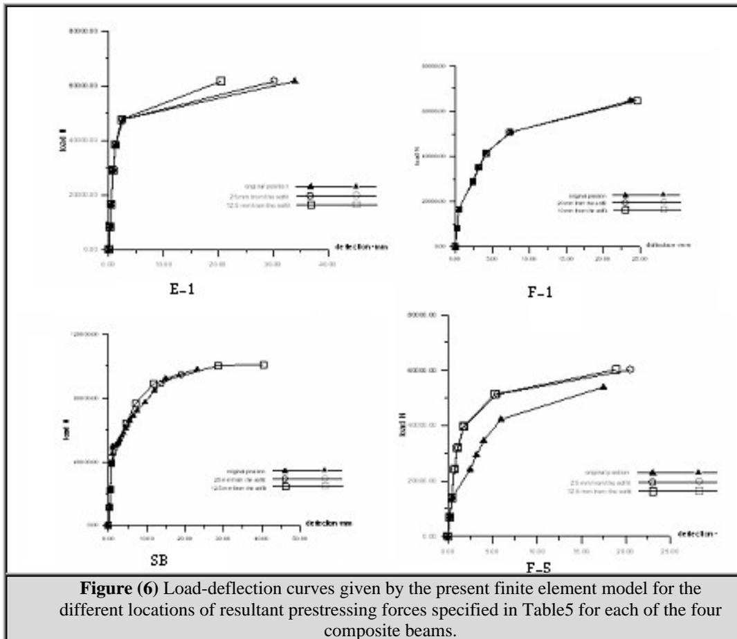
**Figure (6)** Load-deflection curves given by the present finite element model for the different locations of resultant prestressing forces specified in Table5 for each of the four composite beams.
