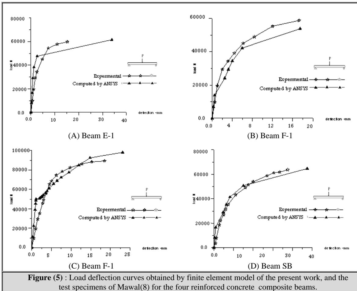
Figure (5) : Load deflection curves obtained by finite element model of the present work, and the test specimens of Mawal(8) for the four reinforced concrete composite beams.
