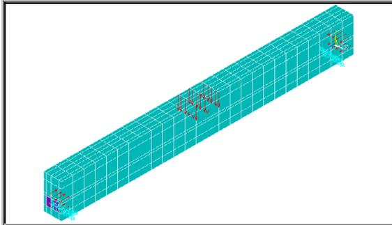
**Figure (3)** Typical finite element mesh pattern simulation of the applied concentrated load, the reactions, and the prestressing forces for each of the four analyzed composite beams.
