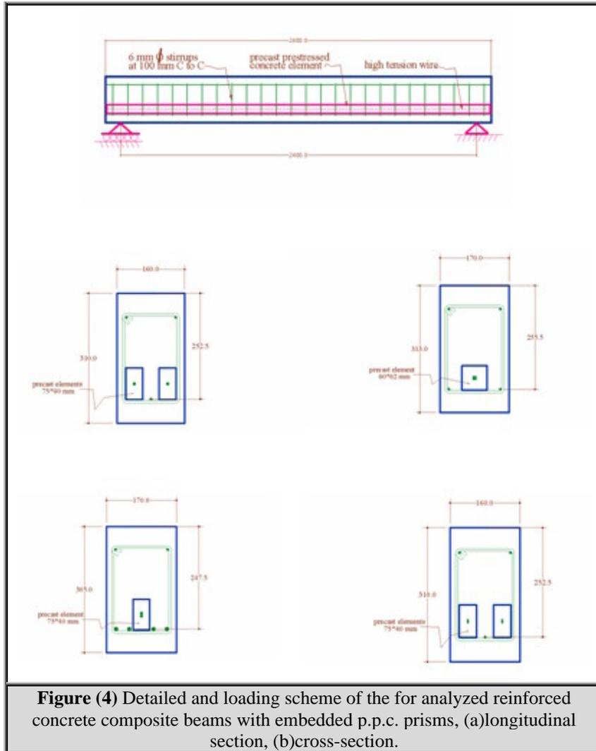
**Figure (4)** Detailed and loading scheme of the for analyzed reinforced concrete composite beams with embedded p.p.c. prisms, (a)longitudinal section, (b)cross-section.
