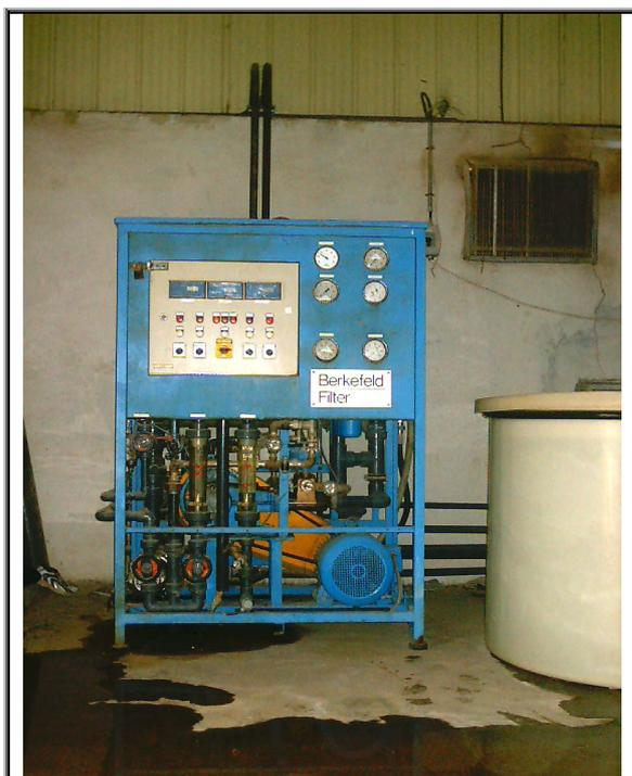
Figure (2) Pilot plant RO unit (Berkefeld Filter).
