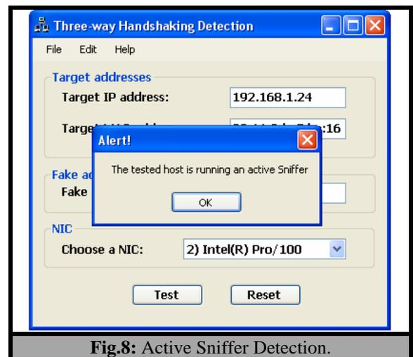
**Fig.8:** Active Sniffer Detection.
