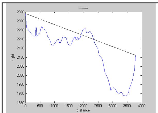
**Figure (14)** Line-of-sight and path profile between points A and B1.
