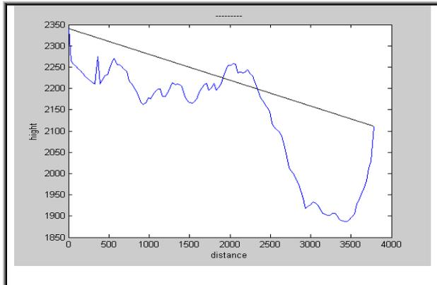
**Figure (17)** The First Fresnel Ellipsoid between the points A and B1.
