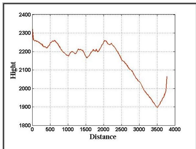
**Figure (16)** Line-of-sight and path profile between points A and B3.
