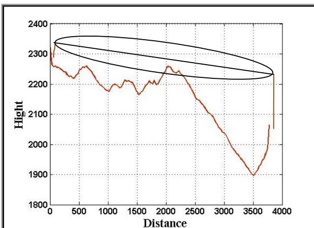
**Figure (19)** The First Fresnel Ellipsoid between the points A and B3.
