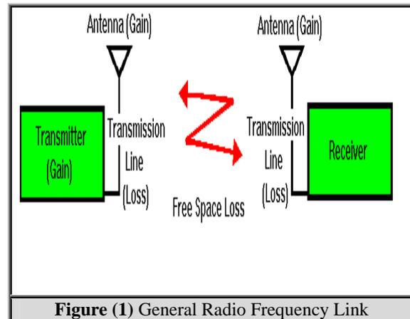
Figure (1) General Radio Frequency Link
