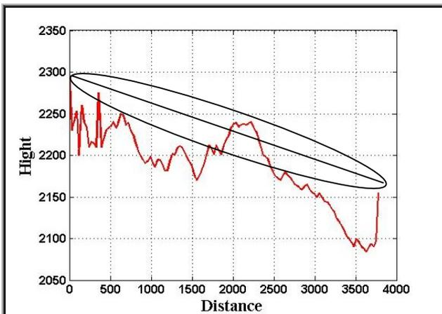
**Figure (18)**. The First Fresnel Ellipsoid between the points A and B2.
