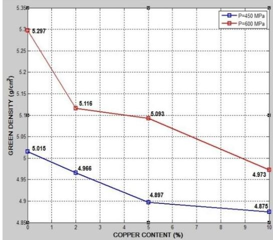
**Figure 4:** Green density as a function of copper content for compacting pressure 450 and 600 MPa.
