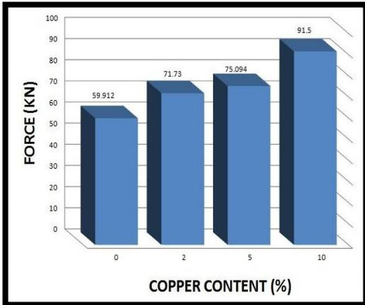
**Figure 11:** Compression failure as a function of copper content for 600MPa.
