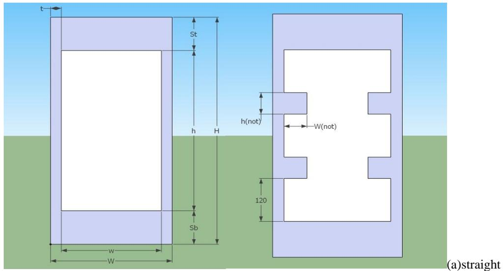
rectangular(b) Microchannel with two-Notches
