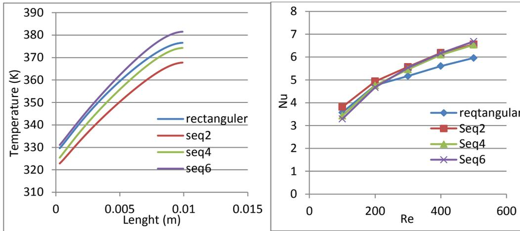
**Figure 9:** Variation on fluid temperature for pure water, at ( $Re=100$ ) & ( $Q=150$ )  $W/cm^2$  at bottom channel wall
