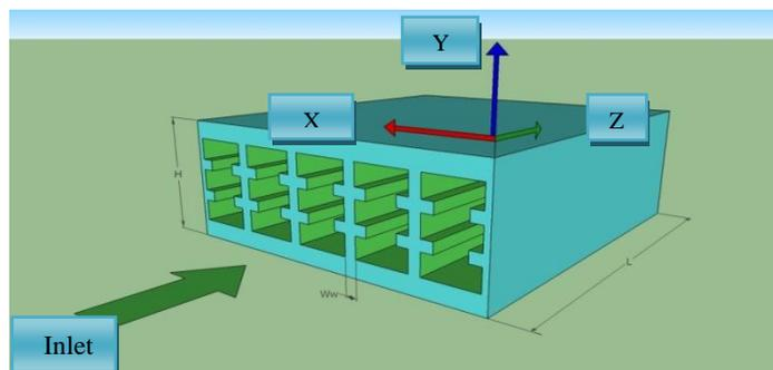
**Figure 1:** Schematic diagram of the microchannels heat sink
