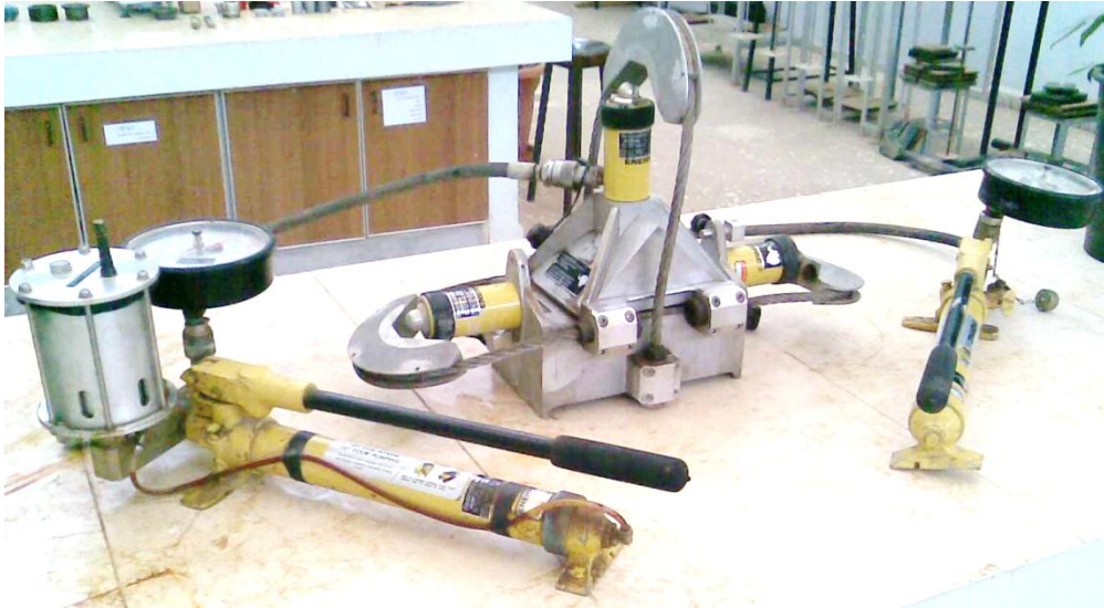
Figure 11: The portable rock shear box apparatus
