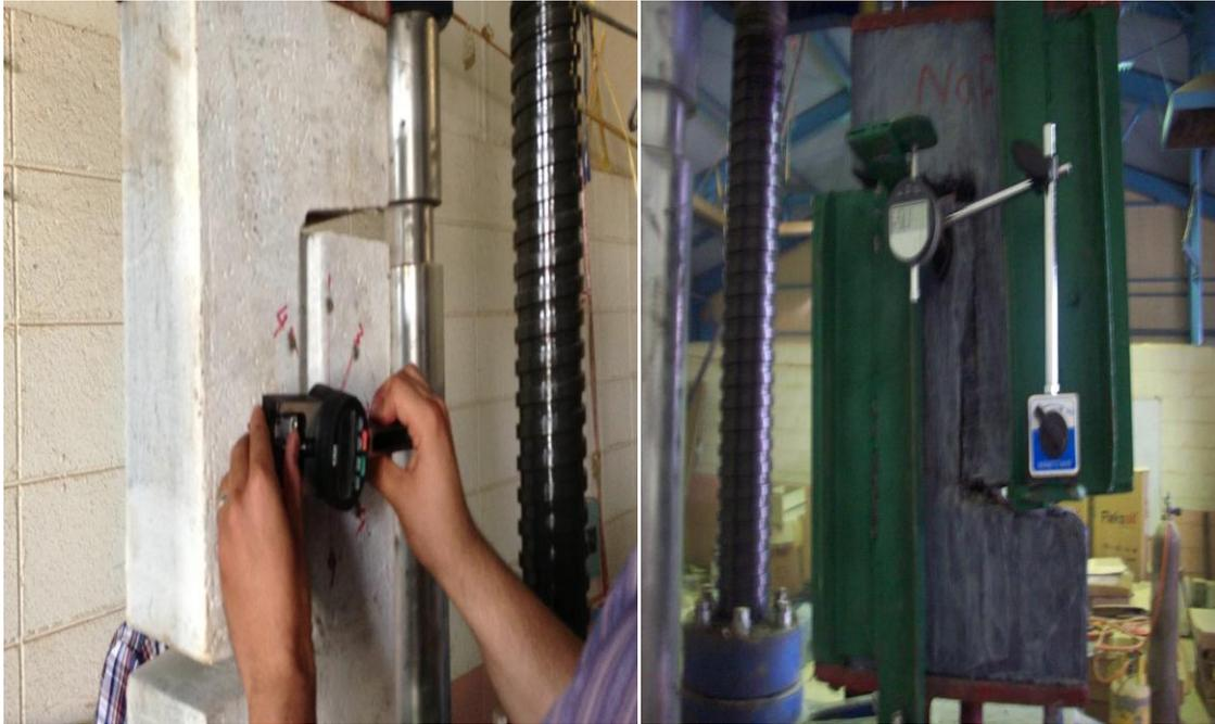
**Figure 3:** Measurement of Deformations
