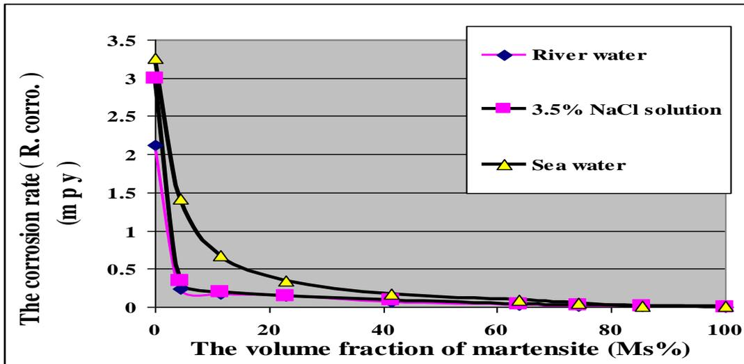
Figure 11: Percentage of volume fraction of martensite (Ms%) vs corrosion rate( $R_{corr.}$ )(m p y) , for different mediums .
