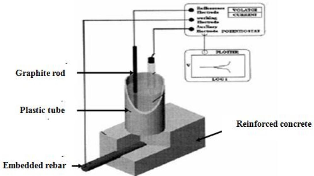
Figure 10: Schematic of the connection between the potentiostat and the three electrodes to the DC corrosion measurement software [11] .
