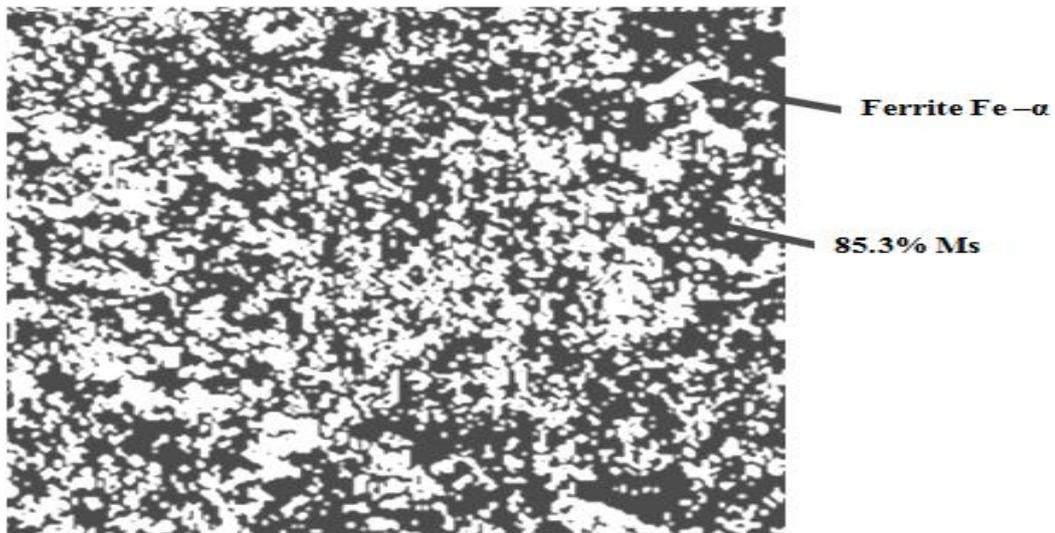
**Figure 8:** The microstructure of the Dual-phase steel ,( 860<sup>0</sup>C) annealing temperature ,( X1000) .
