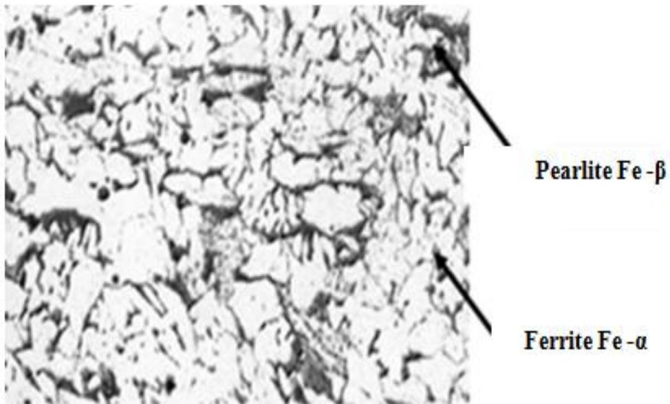
**Figure 2:** The microstructure of the Ukrainian (0.22% C) steel (X200) .
