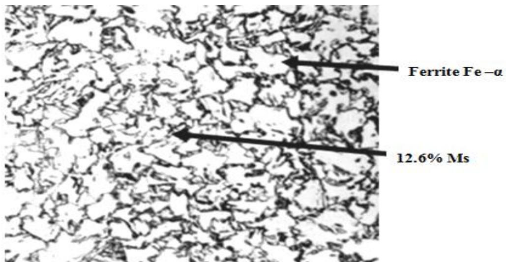
**Figure4:**The microstructure of the Dual-phase steel ,( 760<sup>0</sup>C) annealing temperature , (X500) .
