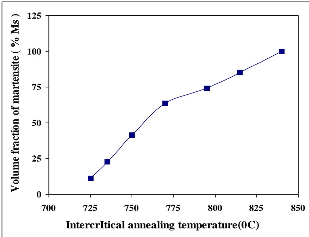
Figure 9: Percentage of volume fraction of martensite vs intercritical annealing temperature (°C) for the Ukrainian (0.22%C) steel .
