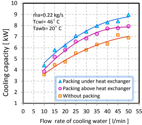
**Figure 21:** Variation of cooling capacity with cooling water flow rate for different locations of packing
