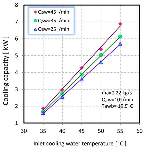
**Figure 11:** Variation of cooling capacity with inlet cooling water temperature for different spray water flow rates
