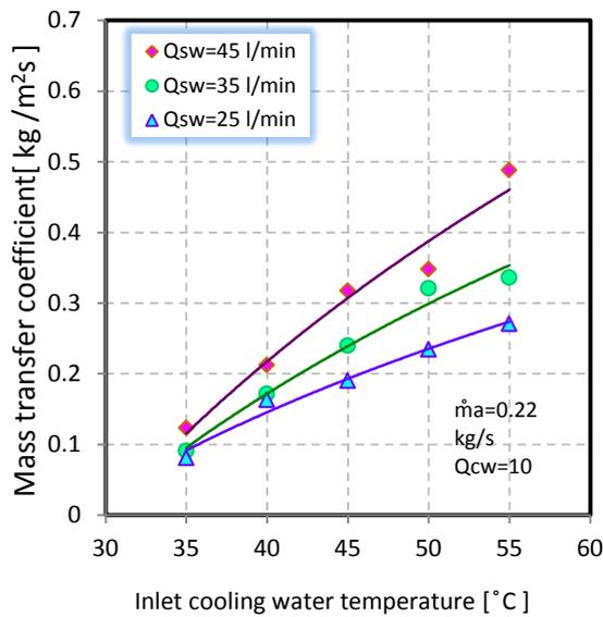
**Figure 13:** Variation of mass transfer coefficient with inlet cooling water temperature for different inlet water temperatures
