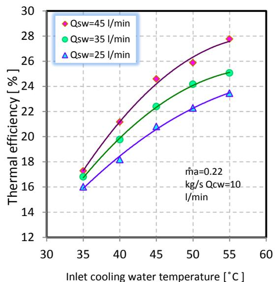
**Figure 12:** Variation of thermal efficiency with inlet cooling water temperature for different spray water flow rates
