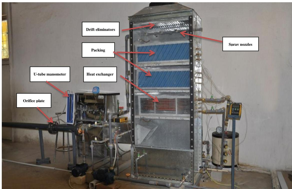
**Figure 1b:** Photographic picture for experimental apparatus (front view)
