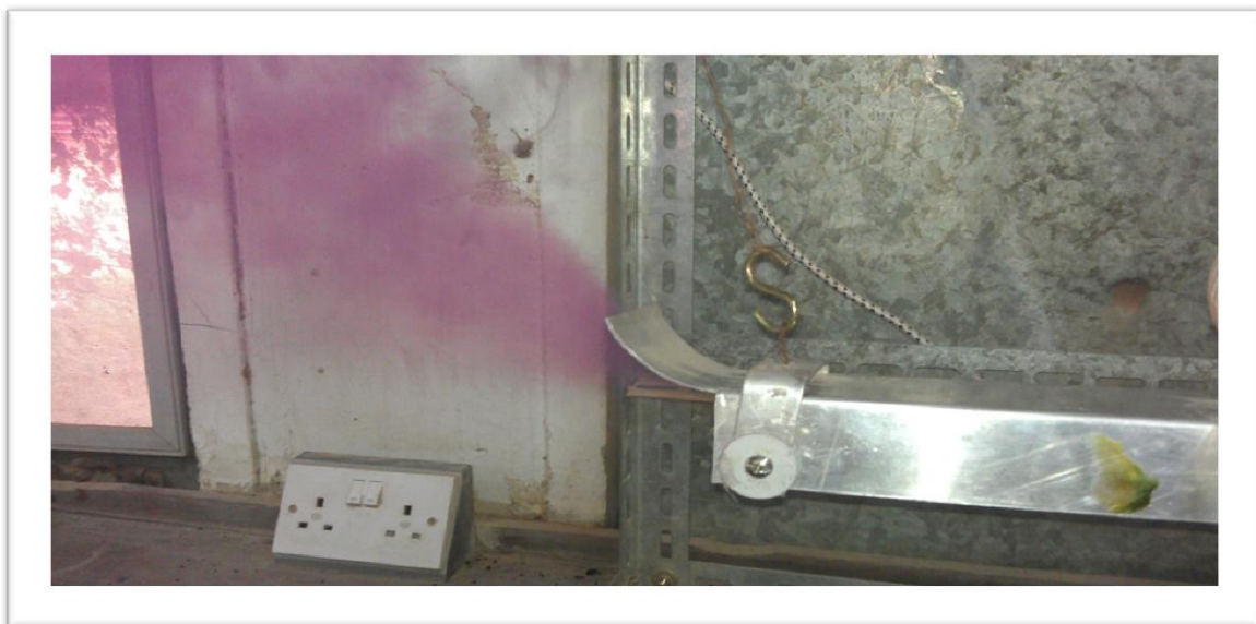
Figure 18: Visualisation of a vectoring primary jet for M_s/M_p=0.2613, g/H=3.53
