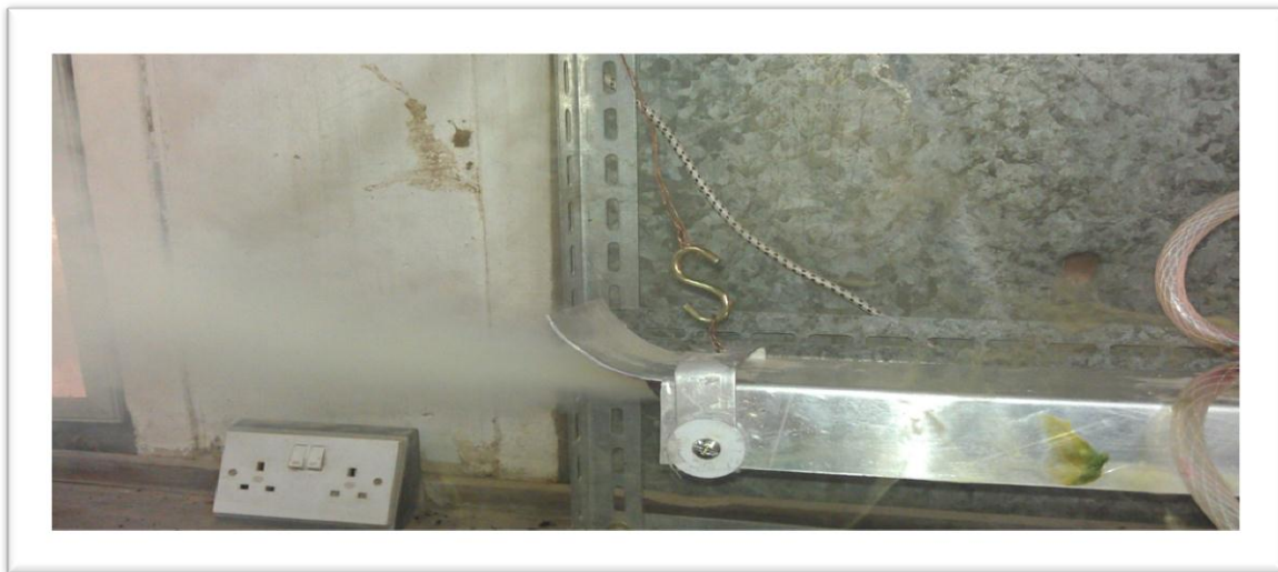
Figure 17: Visualisation of a non-vectoring primary jet for M_s/M_p=0, g/H=2.353 .
