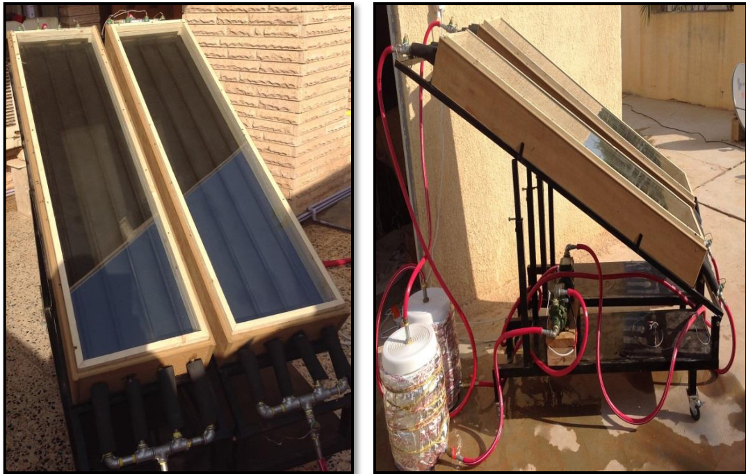
Figure 2: flat plate solar collectors
