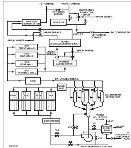
**Figure (1) :water/ steam circuitry**
