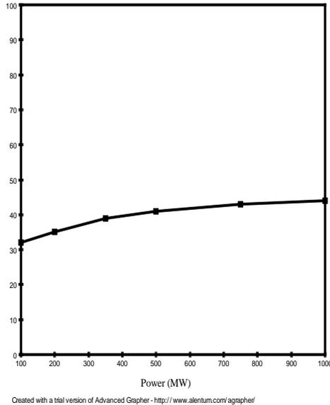
**Figure (13) :** Plant efficiency variation power of plant.
