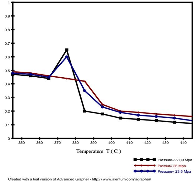
**Figure (7):** Thermal conductivity variation with bulk temperature
