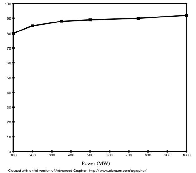
**Figure (12) :** Boiler efficiency variation with power of plant.
