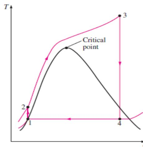
**Figure(3): The T-s diagram of a supercritical Rankine cycle[Yunus 2006]**
