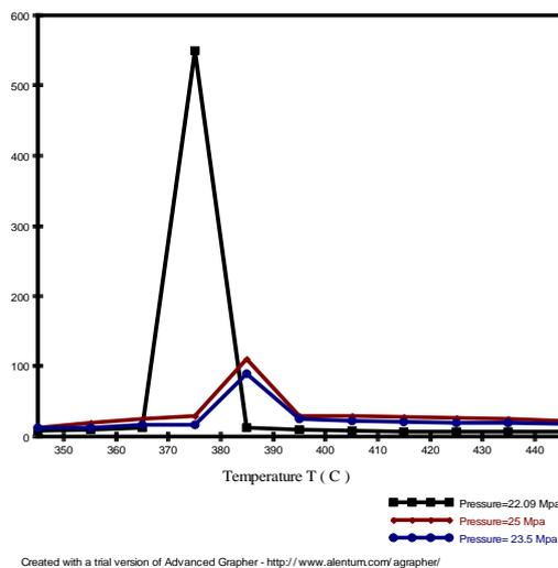
**Figure (6):** Specific heat variation with bulk temperature.
