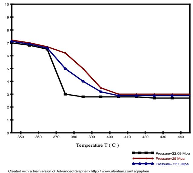
**Figure (8):** Dynamic viscosity variation with bulk temperature.
