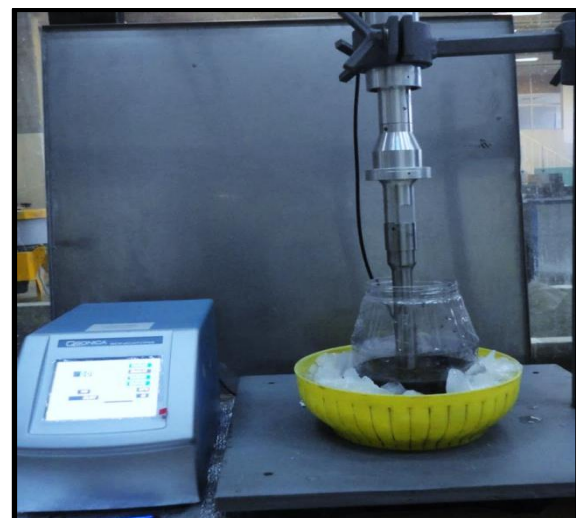
Figure 1: Ultrasonic Liquid Processors Q700 sonicator from QSONICA, LLC. used for CNTs dispersion
